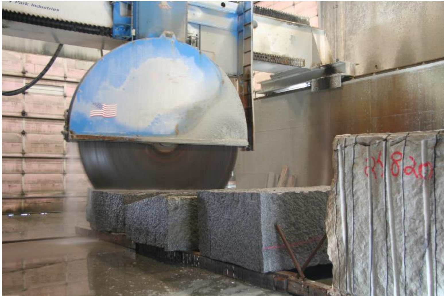
Granite blocks being sawed into slabs at Bedrock Granite Sales processing facility in Coquitlam.
