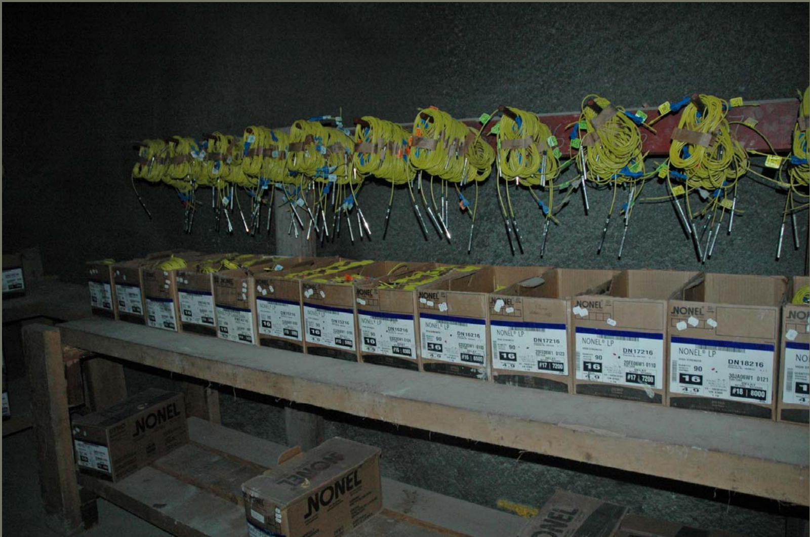
5 - Blasting caps (shiny metal ends) attached to fuses (yellow wires).
