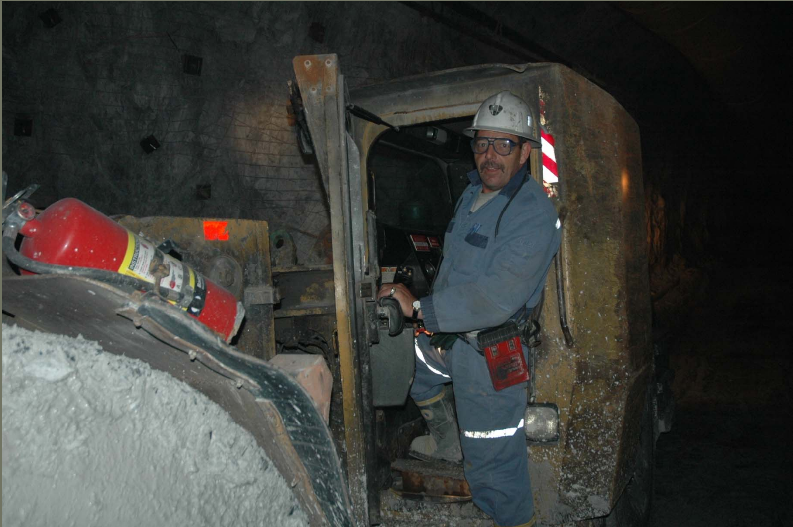
10 – Miner at the controls of a scoop tram.
