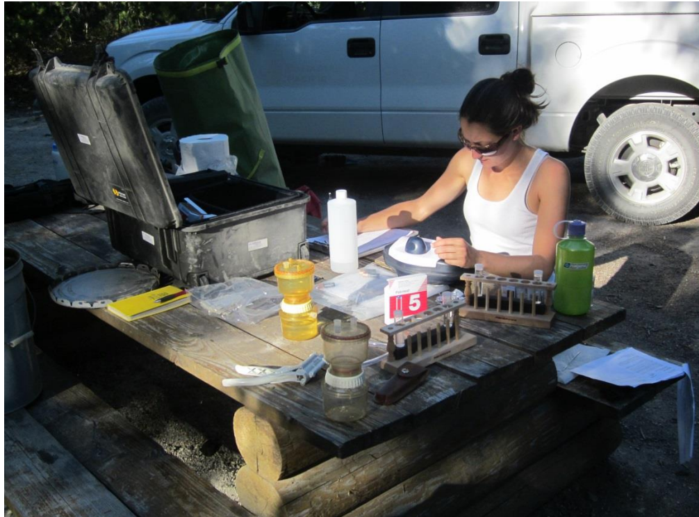
Set-up and equipment needed for Photometer analysis in the field. The Palintest Photometer 8000 is the blue and white device at the bottom right of the picture.
