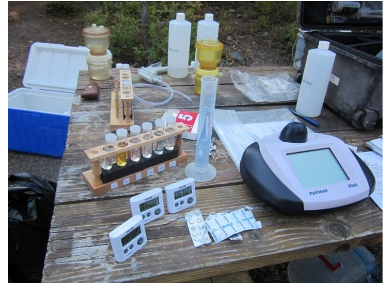
Set-up and equipment needed for Photometer analysis in the field. The Palintest Photometer 8000 is the blue and white device at the bottom right of the picture.
