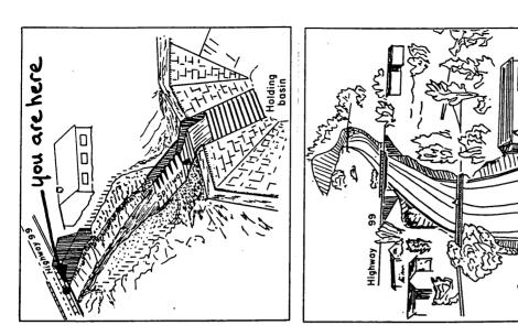
**Figure 2 (a)** Dam, holding basin and spillway (looking downstream) on Harvey Creek, designed to prevent debris flow damage to the community of Lions Bay.
