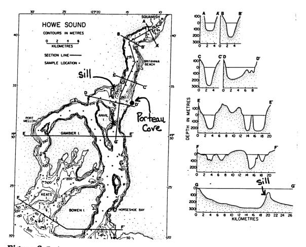
**Figure 6** Bathymetric chart of Howe Sound and topographic profiles (From Syvitski and Luternauer, 1982).
