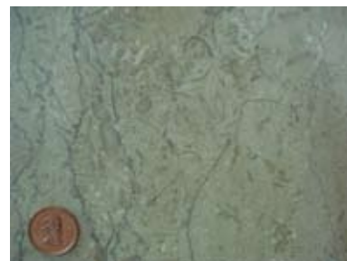
Figure 17 – Fossiliferous limestone with large football-shaped forams and other fossil debris; Vancouver Main Post Office. The dark grey zig zag surfaces are stylolites.
