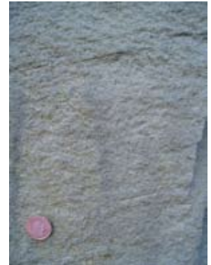
Figure 30 – Sandstone block from the Cathedral showing inclined laminations, some with black organic debris.
