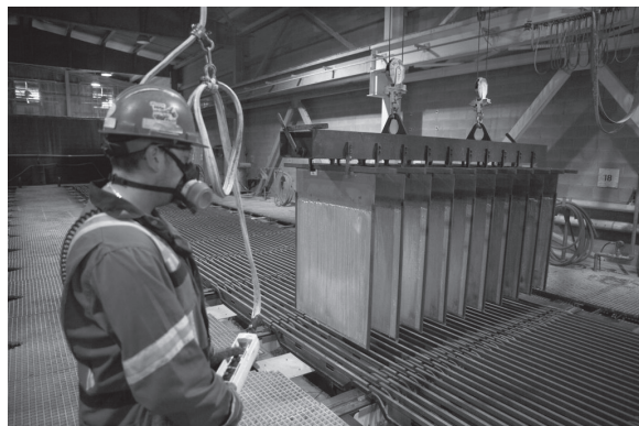
At Gibraltar Mine near Williams Lake, BC copper in oxide minerals is leached in an acidic solution and plated onto aluminum sheets in the on-site SX-EW plant (not in operation in 2009).
