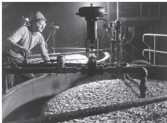
A mill operator inspects the slurry in one of the three flotation cells in the mill at Highland Valley Copper Mine.
