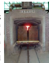
Harrop tunnel kiln for bricks on rail cars, Clayburn Industries.
