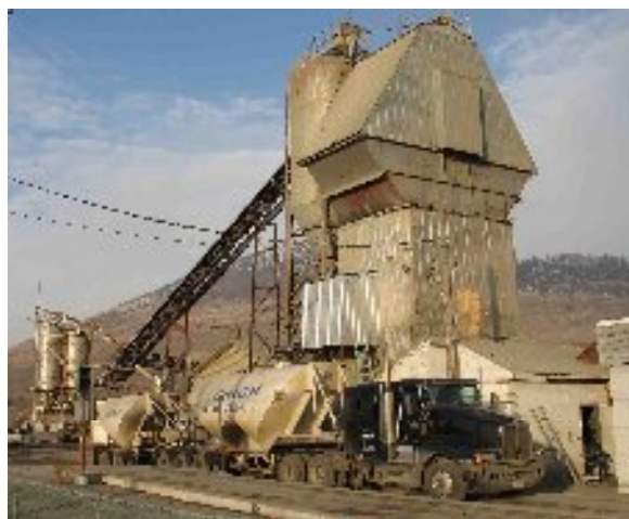
Figure 48. Sand, gravel, cement, additives, and water stored in the tower are carefully measured and mixed at the concrete redi-mix plant. (Photo by R.Turner)
