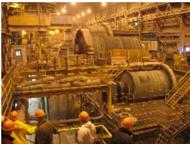
Figure 42. (Left) Large cylindrical mills grind the ore from football size blocks to silt. (Right) Flotation tanks in the mill
