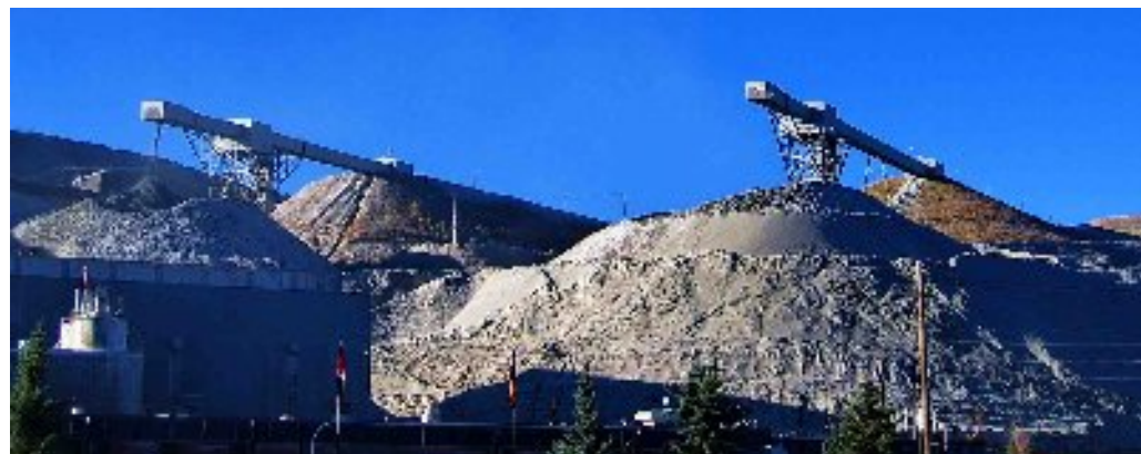
Figure 40. (Left) Conveyor belts carry football size blocks of ore from the pit to stockpiles (centre) at the mill (lower left), ready for processing. (Photo by R. Anderson)
